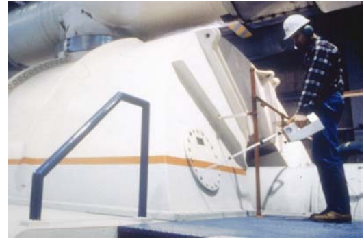
Figure 15 SF6-Pak Hand-held Tracer Gas Dispenser
