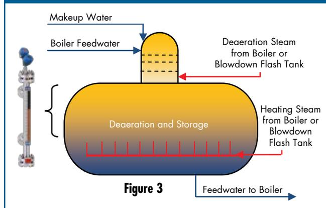
As with any feedwater heater, the level is critical in maintaining a consistent condensing zone to maximize the transfer of energy from the steam to the boiler feedwater while ensuring adequate boiler feedwater reserves are available. Of course, any appreciable gains in boiler feedwater that can be achieved in the deaerator reduces the amount of energy (fuel) required at the boiler – every 10.8°F (6°C) rise in boiler feedwater amounts to a one percent savings in fuel cost.
